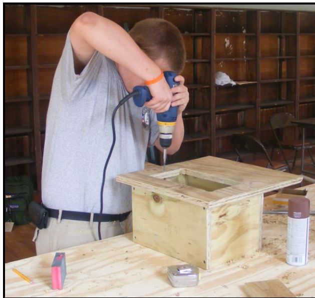
Assemble the sun collar box onto the sun collar platform.
