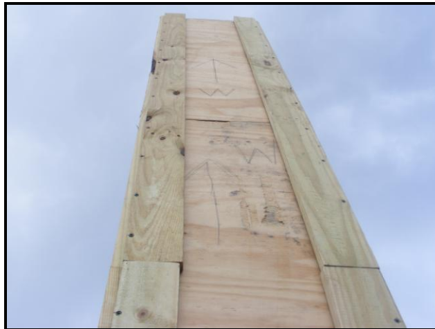
Two assembled nesting chambers with braces. Notice the screws on the far corner of each edge, roughly 1/4" inside.
