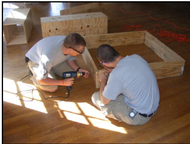
Forming a box out of your cut 2" x 10".
